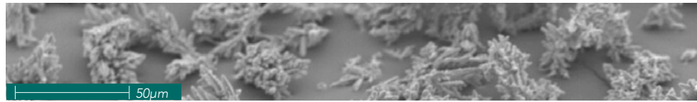
SEM aspect of CU1182 electrolytic copper powder
